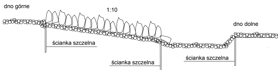
Rys. 5. Schemat modelu bystrza na rzece Khale Fig. 5. Rapid hydraulic structure model on the Khale River
