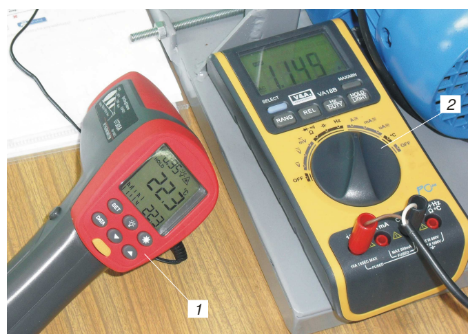
Fig. 3. Temperature and electric motor power measurement devices: 1 – IR Thermometer INI-T UT350A of measuring range -50+1050^{\circ}\text{C} , 2 – digital multimeter V&A VA18B
