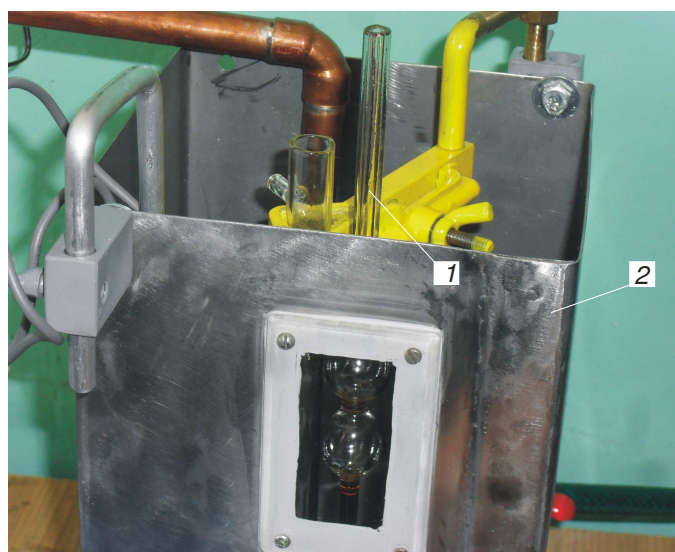
Fig. 4. Pinkiewicz 480 viscosimeter (1) produced by LABIT company mounted in the preliminary oil tank of 5 l volume (2)
